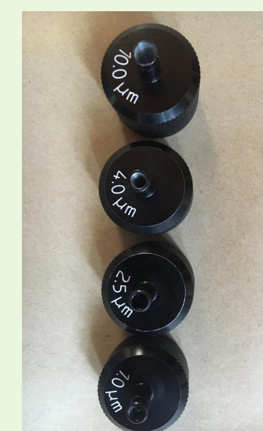
Figure 5. DustTrack for PMs measurements and their impactors.
