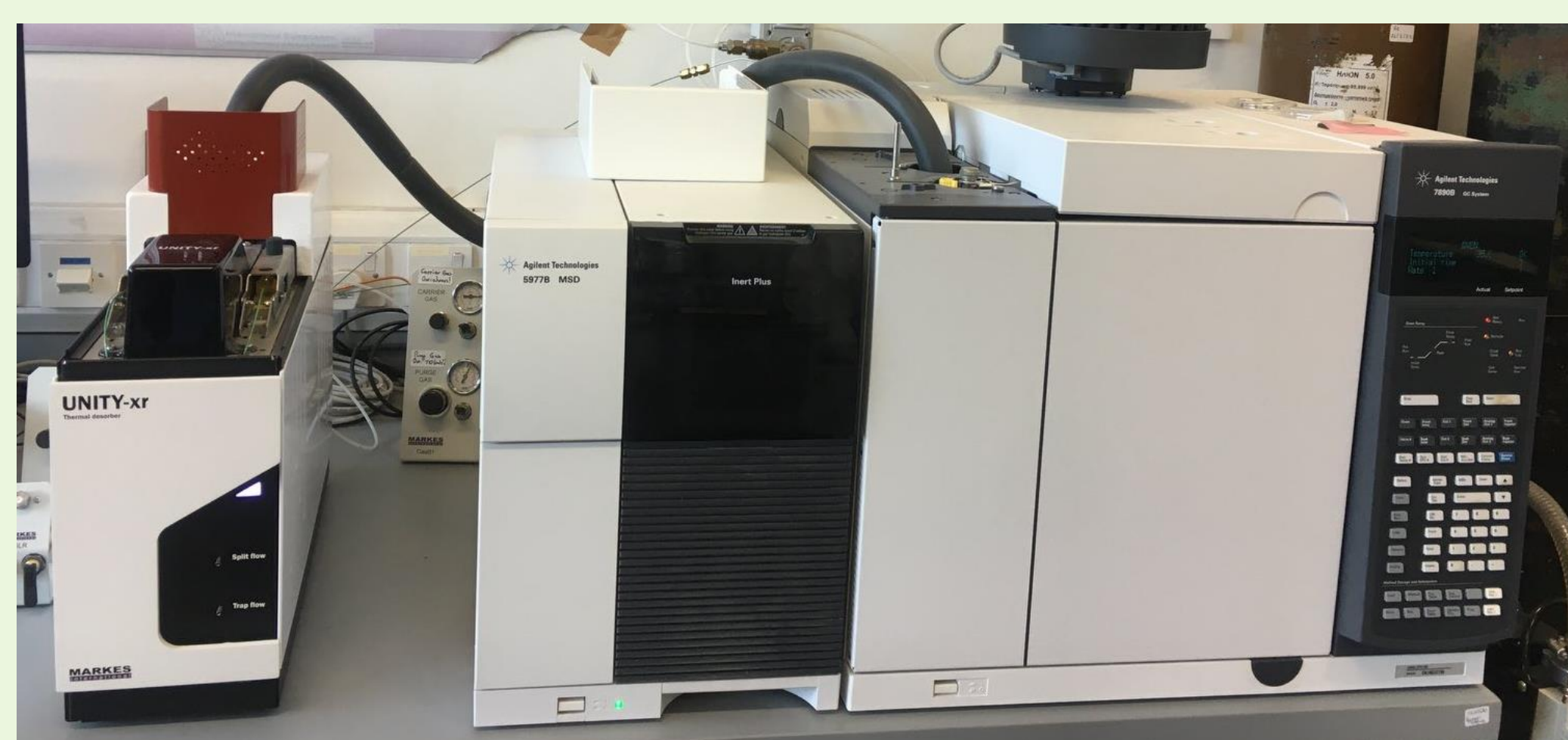
Figure 4. TD-GC/MS system for VOCs analysis.
