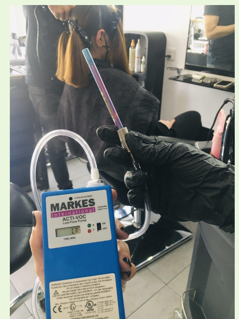
Figure 3. Low-flow pump during on-site sampling.
