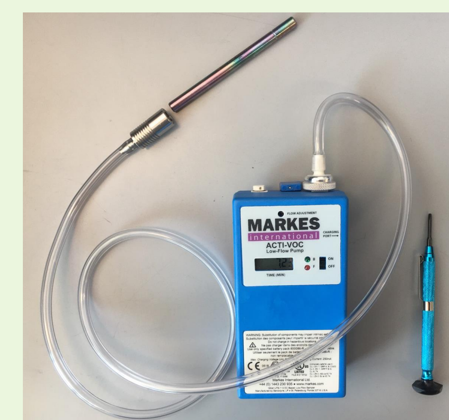
Figure 3. Low-flow pump during on-site sampling.
