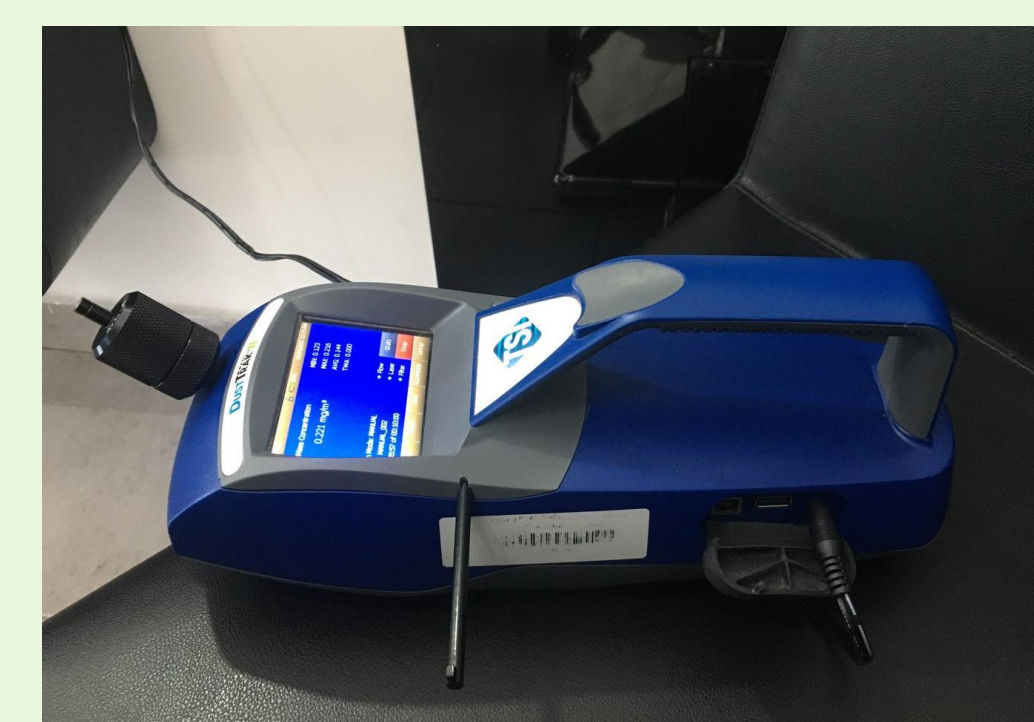
Figure 5. DustTrack for PMs measurements and their impactors.
