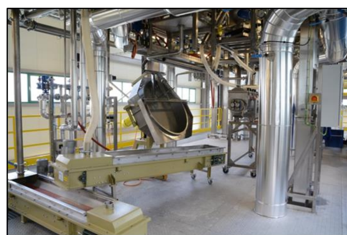
Fig. 2 Installation 1/2 technical scale for the production of microbiologically enriched fertilizers
