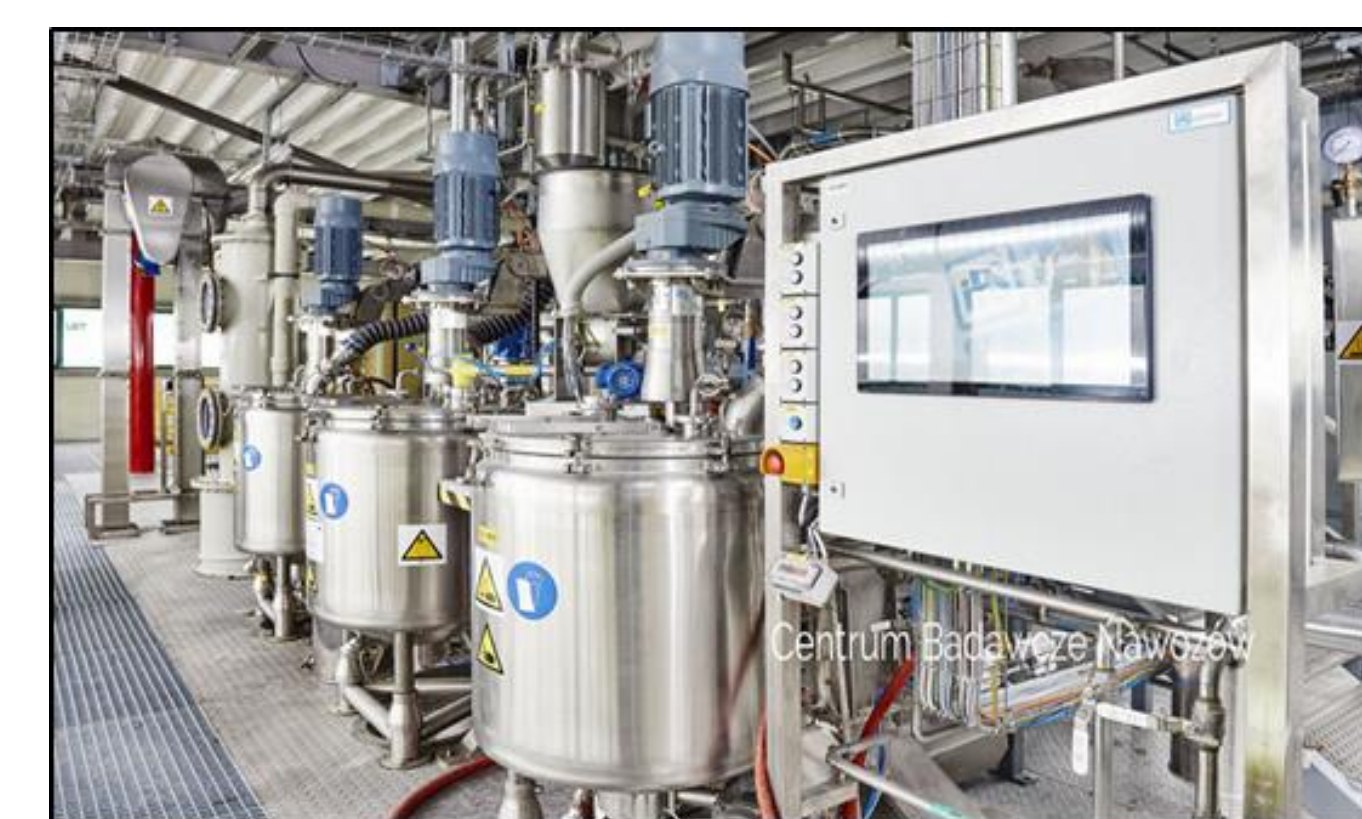
Fig. 2 Installation 1/2 technical scale for the production of microbiologically enriched fertilizers
