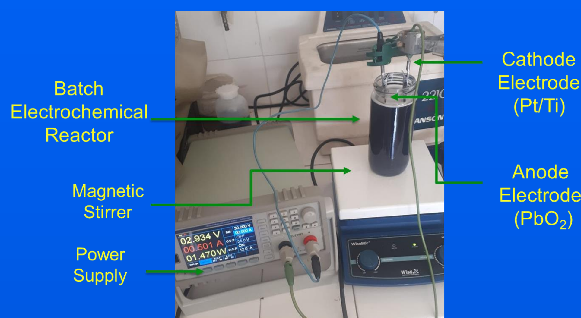
Figure 1: Electrochemical Batch Reactor for Cr conversion
