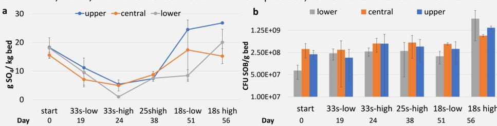
**Figure 3.** Sulfate production (a) and SOB abundance (b) in each biofilter section at different EBRT (33,25 and 18s) and level of gas concentration (high and low). "Day" indicates the biofiltration day of sampling
