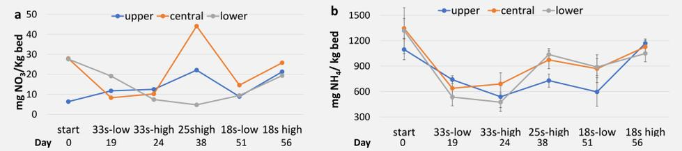
**Figure 4.** Nitrate production (a), ammonium accumulation (b) and AOB abundance (c) in each biofilter section at different EBRT (33,25 and 18s) and level of gas concentration (high and low). "Day" indicates the biofiltration day of sampling
