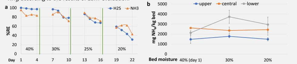
**Figure 5.** Removal efficiency of H<sub>2</sub>S and NH<sub>3</sub> (a), ammonium accumulation (b), sulfate production (c) and SOB abundance (d) in each biofilter section at different moisture content of biofilter bed.
