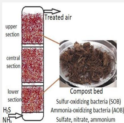
**Figure 1:** Compost based biofilter. Height: 0.81 m, Volume: 0.007 m<sup>3</sup> (6.6 L)
