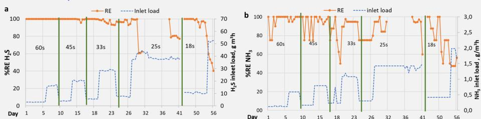
**Figure 2.** Biofiltration of (a) H<sub>2</sub>S and (b) NH<sub>3</sub> under transitory conditions of inlet gas load. From day 32 to 38 there was a shutdown in operation (air compressor failed). %Removal efficiency (%RE) in orange line. Numbers inside correspond to EBRT. Green lines indicate change of EBRT
