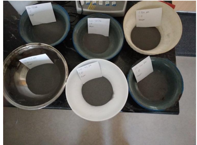
Figure 5. Different particle size fractions of iron powder
