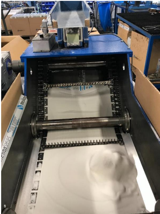
Figure 6. The industrial size aero-suspension separator Figure 6 left. Top view of the machine with charge Figure 6 right. Copper-aluminium scrap for a separation test
