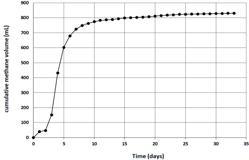
**Figure 1** – Example of raw cumulative methane volume data generated by AMPTS II system during mesophilic digestion of food waste
