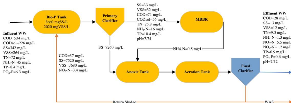
**Figure 2.** Pilot plant layout and the mass balance obtained in the HAS-MBBR configuration
