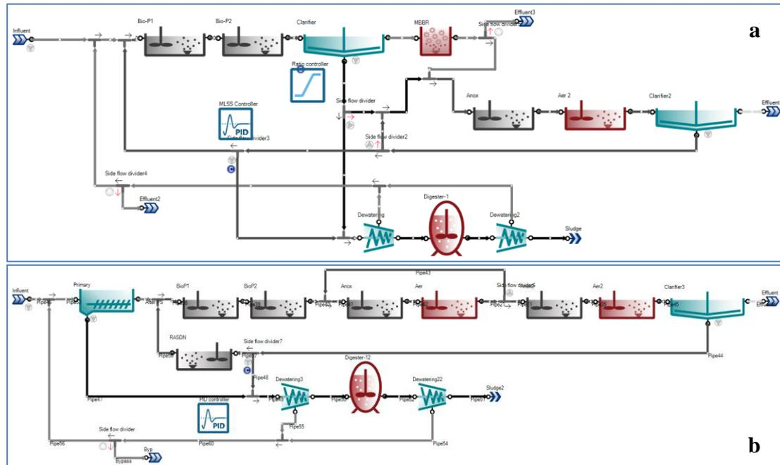
**Figure 1.** Sumo layouts for (a) HAS-MBBR (b) CBNR
