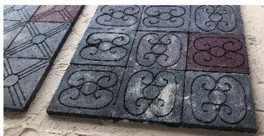
**Figure 1:** Paving blocks from plastic bonded sand (PBS) produced in Gambia.
