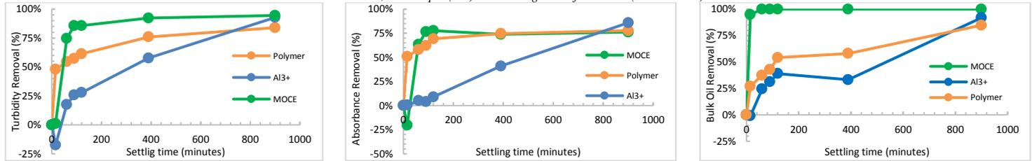
Figure 2: Settling time vs turbidity removal (a.), absorbance removal (b.) and oil removal (c.). Experimental conditions coagulant dosage  $Al^{3+}$  10mg/L, polymer 2.5mg/L, MOCE 50mg/L and initial pH of 7.8
