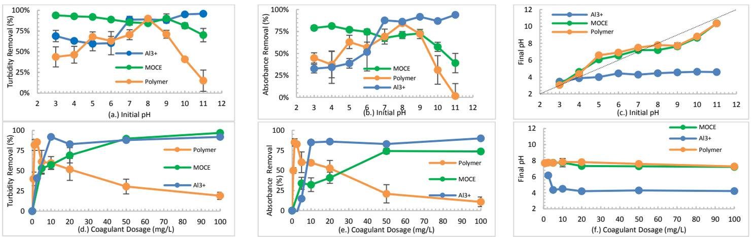
Figure 1: Initial pH vs turbidity removal (a.), absorbance removal (b.), final pH (c.). Experimental conditions, coagulant dosage  $Al^{3+}$  10mg/L, polymer 2.5mg/L, MOCE 50mg/L and settling time of 15 hours (900 minutes). Coagulant dosage vs turbidity removal (d.), absorbance removal (e.) and final pH (f.). Experimental conditions, neutral pH (7.8) and settling time of 15 hours (900 minutes)
