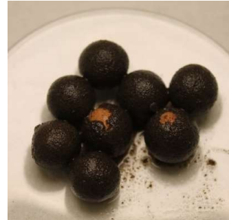
Figure 4: low mechanical resistance of fertilizer coating in water
