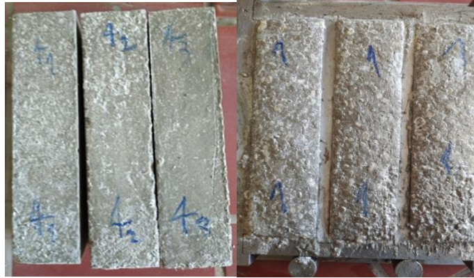
Figure 5: Reference sample without expansion (Left), semiconductor (SC) sample with air bubbles and expansion (Right)
