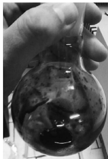
Figure 2. Flask with collected pyrolytic oil
