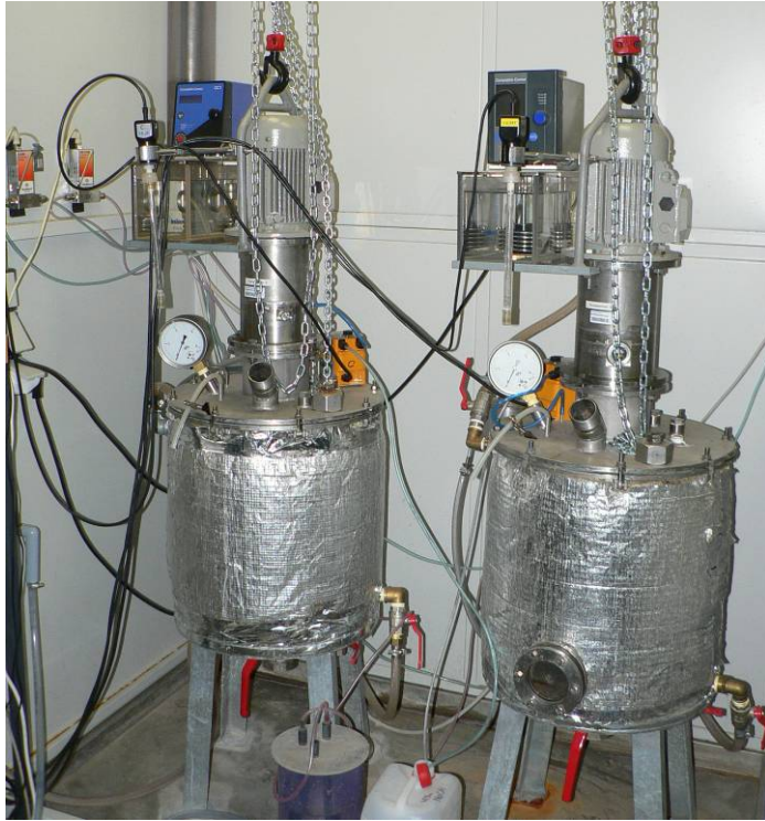
Fig. 2 Photo of the anaerobic laboratory digesters
