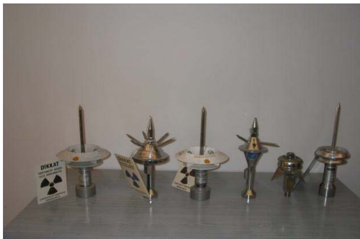
Lightning rods: Am-241, (2-1000 MBq), Ra-226 (4-400 MBq)
