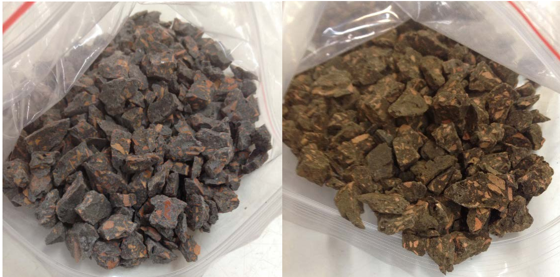
Figure 2: Leaching tests: PC and CAC crushed mortar samples at 28 days
