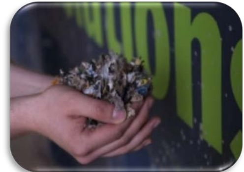
MBT-derived (bio-drying) SRF in the UK, mainly for cement kilns
