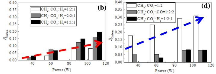
B(c) increased with the increase of discharge power. It means that it will produce more non-CO products at higher discharge power.
