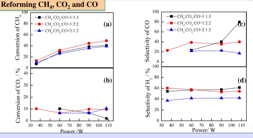
The addition of CO into  $CH_4$  and  $CO_2$  in the plasma reforming process would inhibit the conversion of  $CO_2$  (b), however, it had tiny influence on the conversion of  $CH_4$  (a). It can be concluded that  $CO_2$  might have the unique transformation paths, however,  $CH_4$  might have non-unique transformation paths.
