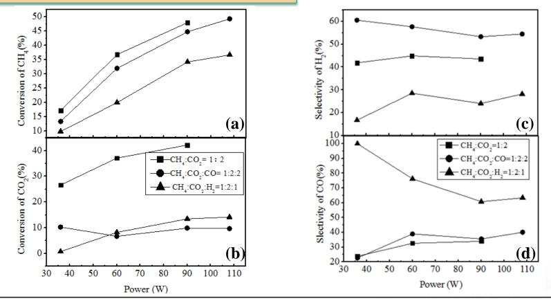
The conversion of  $CH_4$  increased with the discharge power increasing, whereas the addition of CO and  $H_2$  had tiny influence on the conversion of  $CH_4$  (a).
