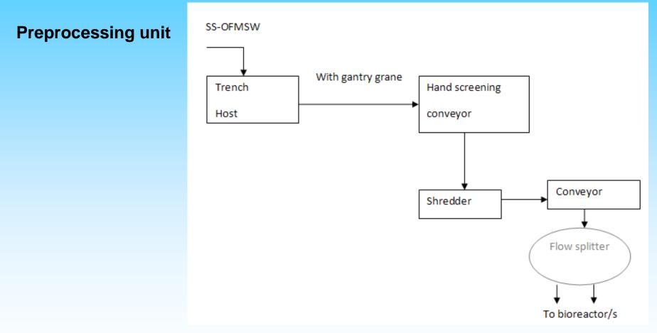
a trench host (capacity 122-140m3), gantry crane for transferring material from the trench in hand screening conveyor, shredder and a conveyor that will lead the product in the bioreactor/s
