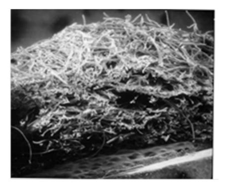
Cross section of barrier of regenerated waste fibers obtained by the wet process
