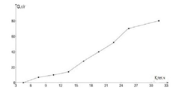
Influence of wool content in the mixture with polyester on the retention of oil and petroleum products. The filter barrier of recycled fibers has a stable structure, air permeability coefficient Bp =  $0.803-1.22 \text{ m}^3/\text{m}^2$ .h, distribution of pore size of 212- 240 µm, an average pore size of about 226 µm, with an average thickness - 12 to 15 mm and area density 250 g/m<sup>2</sup>, with an average dry and wet breakthrough strength respectively 13.15 dN and 10.65 dN.
