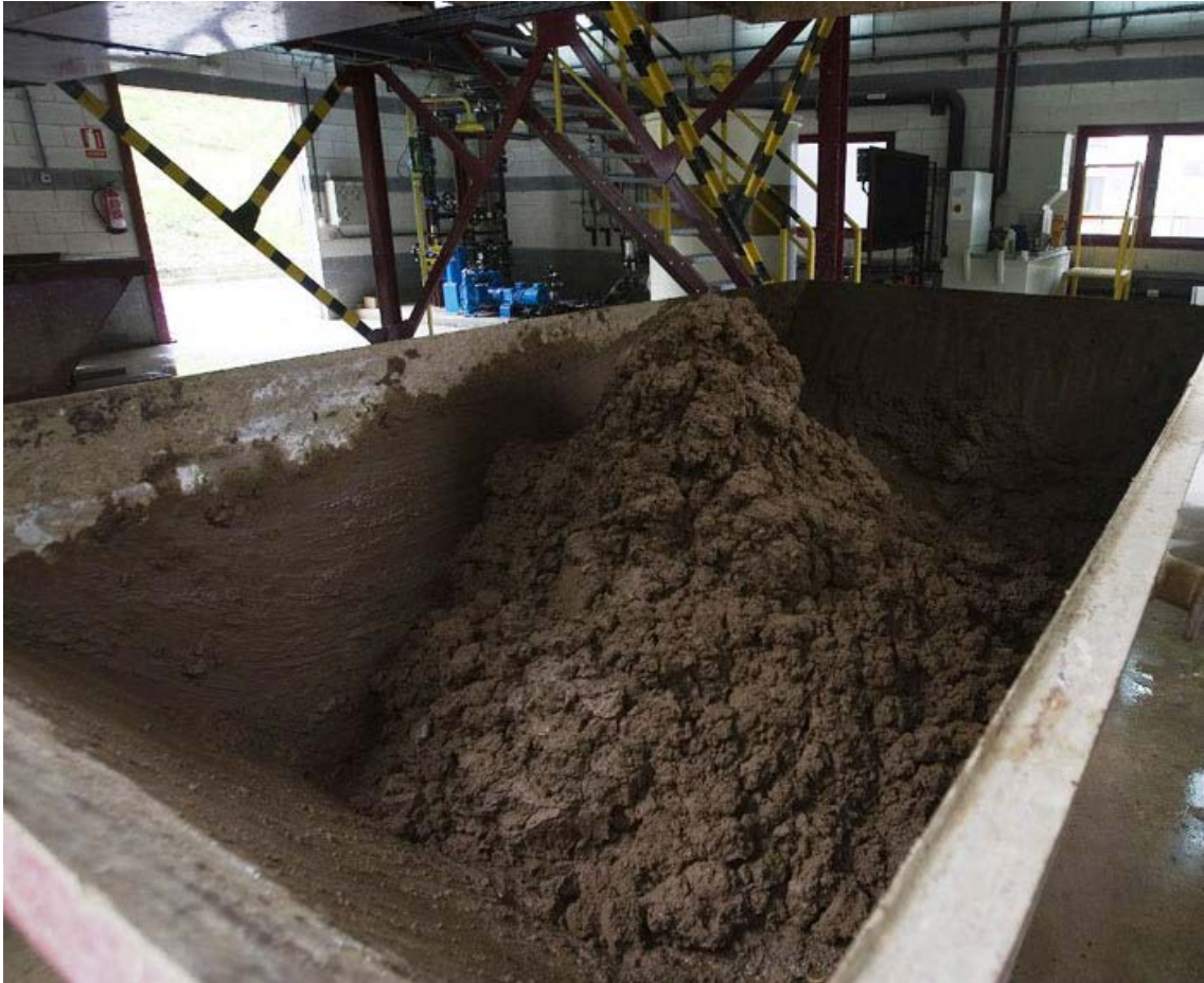
Fig. 1. Sewage sludge from WWTP which daily production is equivalent to 1 kg per inhabitant. It is a hazardous waste.
