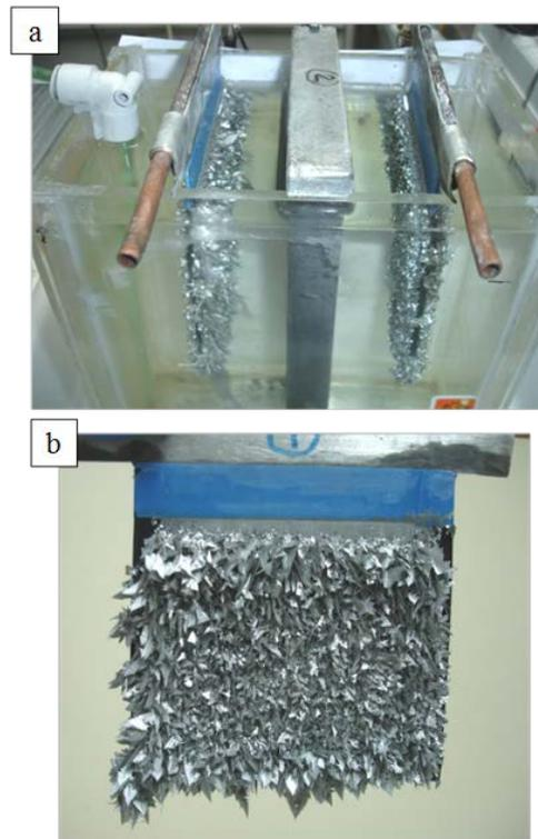
Figure 6. Tin deposits resulting in the electrorefining of alloy 3.
