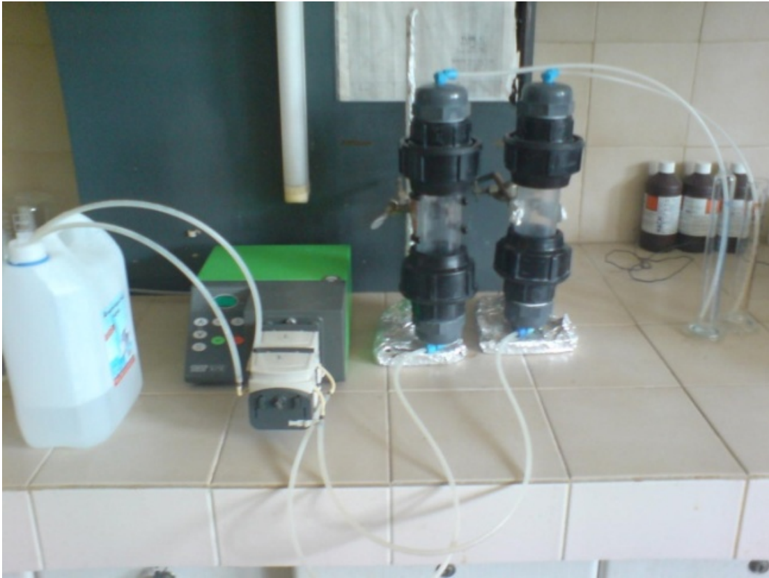
Figure 1. Experimental setup for the dynamic leaching test prEN 14405.
